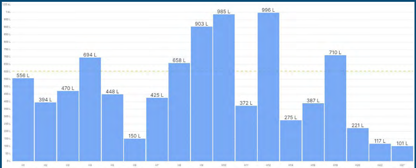
Smart Neighbourhood Pilot Project: Daily average water use per household. The dotted orange line represents the Perth average water use per household (604 litres/household/day).
